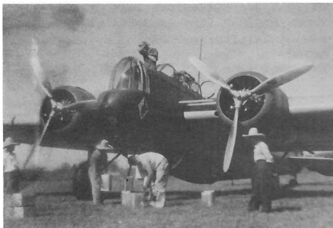
Martin B-10 of 28th Bomb Squadron at unidentified emergency field, 1938. Quantities of gas and other supplies were kept at these fields. Tins were loaded by hand into airplane. (George Tweedy)
